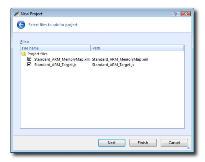
The **Project files** group shows the files that will be copied into the project. The only files used are the memory map file, which describes the memory layout used by the application, and the script used to reset and control the target. For the debugging session to work correctly, each of these files must match and be appropriate for the application you are debugging.
