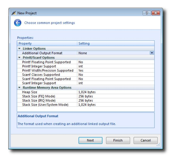
Here you can customize the project by altering a number of common project properties, such as an additional file format to be output when the application is linked and what library support to include if you use **printf** and **scanf**. After the project is created, you can change these settings in the Project Explorer as needed.
