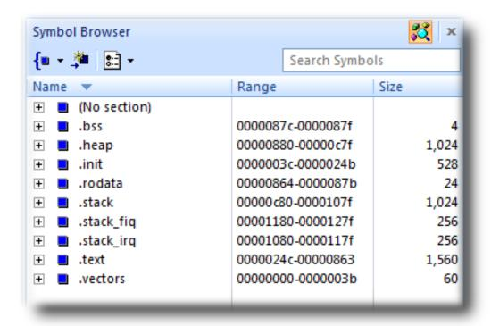
From this, you can see sections and their sizes. For example, the .vectors section containing the ARM exception vectors is placed in memory between address 0x00000000 and 0x0000003B.
