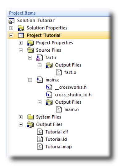
In the above figure, we can see that the files fact.o and main.o are object files, produced by compiling their corresponding source files. The linker script Tutorial.ld, the map file Tutorial.map, and the linked executable Tutorial.elf are produced by the linker. As a convenience, double-clicking an object file or a linked executable file in the **Project Explorer** will open an editor showing the disassembled contents of the file.
