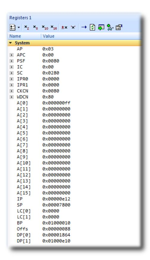
You can also use the registers window to display peripheral registers. To display the state of the target's GPIO registers, select **GPIO** from the **Register Groups** menu.
