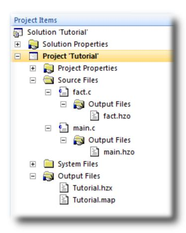
In the above figure, we see that the object files fact.hzo and main.hzo are object files produced by compiling their corresponding source files; the map file Tutorial.map and the linked executable Tutorial.hzx are produced by the linker. As a convenience, double-clicking an object file or a linked executable file in the **Project Explorer** will open an editor showing the disassembled contents of the file.
