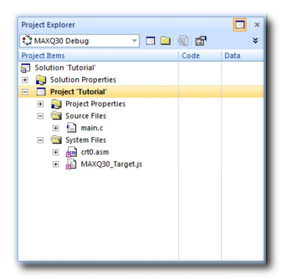
The project name is shown in bold to indicate it is the active project (and, in our case, the only project). If you have more than one project, you can set the active project by using the drop-down box on the **Build** tool bar or by right-clicking the desired project's name in the **Project Explorer** to display the shortcut menu with the **Set as Active Project** command.
