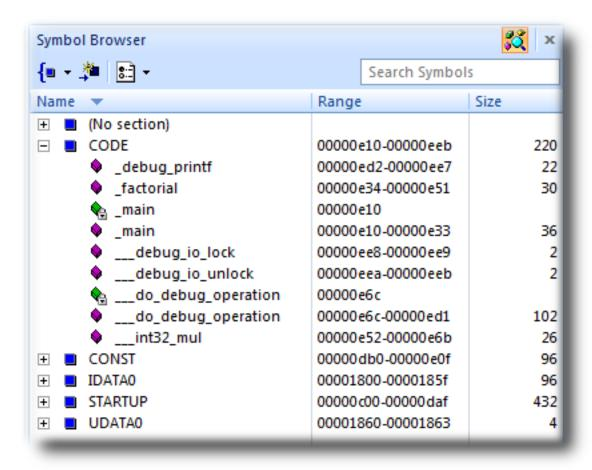
Here, we can see that **main** is 36 bytes in size and is placed in memory between addresses 00000E10 and 00000E33, inclusive, and that **factorial** is 30 bytes and occupies addresses 00000E34 through 00000E51. Just as in the **Project Explorer**, if you double-click a function, CrossWorks moves the cursor to the line containing the definition of that function, so you can easily use the **Symbol Browser** to navigate around your application.
