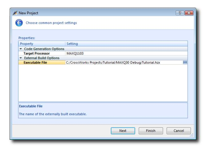
In the Executable File field, type the path to the Tutorial.hzx executable file we generated earlier. For example, if the project was created in the C:/CrossWorks Projects/Tutorial directory and was built using the MAXQ30 Debug configuration, the path to the executable file will be C:/CrossWorks Projects/Tutorial/MAXQ30 Debug/Tutorial.hzx.
