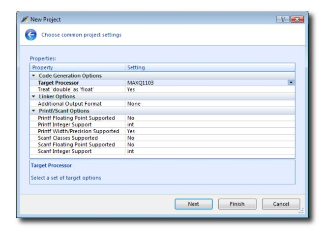
Here you can customize the project by altering a number of common project properties, such as an additional file format to be output when the application is linked and what library support to include if you use **printf** and **scanf**. After the project is created, you can change these settings in the Project Explorer as needed.
