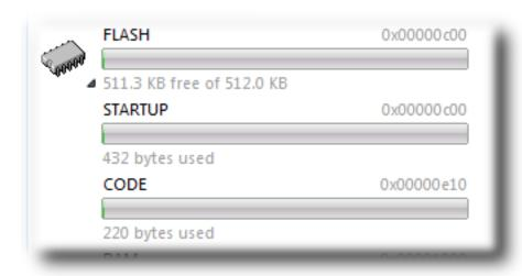
From this, you can see that the the CODE section is located at 00000E10 and is 220 bytes in length.
