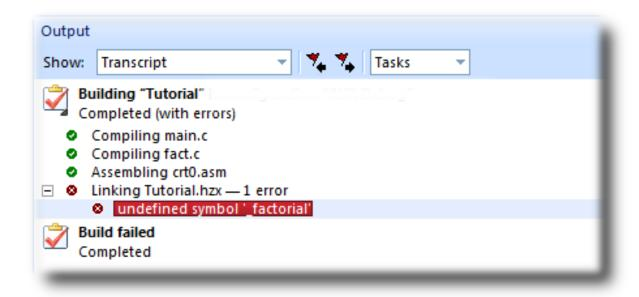
The remaining error is a linkage error. Double-click fact.c in the **Project Explorer** to open it for editing and change the two occurrences of fact to factorial. Rebuild the project—this time, the project compiles correctly:
